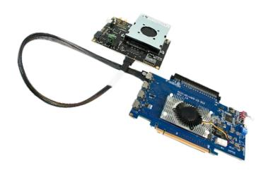
Connect to a compatible MCIO host card, removing the need for adaptors or a U.2 host.
