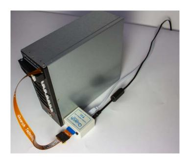
Control a single breaker module via USB or Serial.
