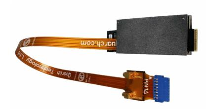
Optional triggering version has MCX trigger in/out.
