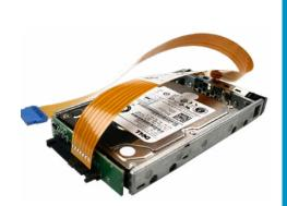
**LITE BREAKER:** FET SWITCHES ON POWER RAILS, DIGITAL SWITCHING ON SIDEBANDS. HIGH SPEED LANES AND GROUNDS ARE PERMANENTLY CONNECTED. 1MS TIMING RESOLUTION ON HOT-PLUG SIMULATION. BASIC HOT-PLUG ONLY, NO PIN-BOUNCE, DRIVING OR GLITCH. VOLTAGE MONITORING ON SELECTED RAILS.
