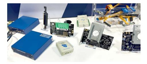
The Torridon system is modular and made up of 'controllers' that run the system and 'breaker modules' that sit in the interface under test.
