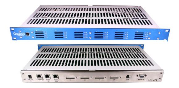
28-PORT CONTROLLER: CONTROLS 28 BREAKER MODULE ACROSS EITHER: DIRECT USB, LAN OR DIRECT RS-232 VIA RS232-D WIRED RJ-45 PORT. 24 PORTS ON FRONT, 4 PORTS ON REAR. 12V 60W SUPPLY. RACK MOUNTS IN 1U. ADDITIONAL USB PORT ON FRONT
