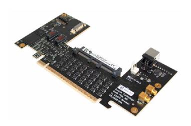
Supports EDSFF devices up to x16. Versions available with lower lane widths.
