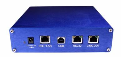
USB, LAN and RS232 Serial control ports.
