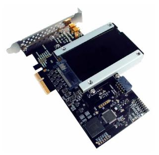
Supports PCle U.2 drives up to Gen5 speeds in a PCle x4 slot.
