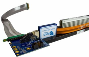
EDSFF PAM: ANALOG CHANNELS: 12V, 3.3VAUX, SAMPLE RATE 250KS/S, VOLTAGE:  $0-15V\pm(2mV+1\%)$ , 12V CURRENT: 100uA-1mA  $\pm$  (25uA+1%) 1mA-13A  $\pm$  (2mA+1%), 3.3VAUX CURRENT: 100uA-85mA  $\pm$  (25uA+1%) DIGITAL CHANNELS: PRSNT0#, PERST1#\_CLKREQ#, LED, SMBRST#, SMBDAT, SMBCLK, PWRDIS, PERST0#, DUALPORTEN#, RFU, MFG, SAMPLE RATE 1MS/S
