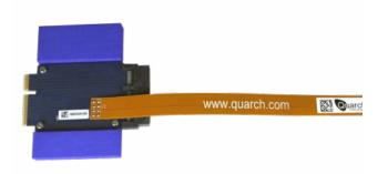
Interposer and flex cable allows power testing within a standard EDSFF enclosure.
