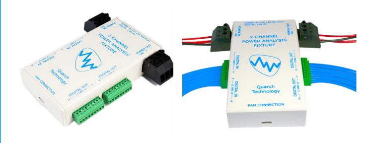
2 CHANNEL: ANALOG CHANNELS: 2 CHANNELS, SAMPLE RATE 250KS/S, VOLTAGE:  $0 - 15V \pm (2mV + 1\%)$ , CURRENT:  $0-1mA \pm (15uA + 1\%) \pm 13A \pm (2mA + 1\%)$  DIGITAL CHANNELS: 16 CHANNELS SAMPLE RATE 1MS/S, VOLTAGE RANGE 1.8-5V
