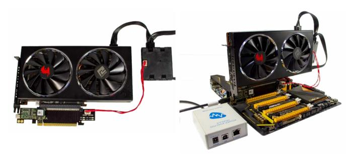
AIC +AUX PAM: ANALOG CHANNELS: 12V, 3.3V, 3.3VAUX, 12VAUX, SAMPLE RATE 250KS/S, VOLTAGE:  $0 - 15V \pm (2mV + 1\%)$ , 12V CURRENT:  $0 - 32.5A \pm (5mA + 1\%)$ , 3.3V CURRENT:  $0 - 13A \pm (2mA + 1\%)$ , 3.3VAUX CURRENT:  $0 - 3.25A \pm (0.5mA + 1\%)$ , 12VAUX CURRENT:  $0 - 162.5A \pm (25mA + 1\%)$  DIGITAL CHANNELS: PERST#, CLKREQ#, WAKE#, SMBCLK, SMBDAT, REFCLK\_LOS#, SAMPLE RATE 1MS/S
