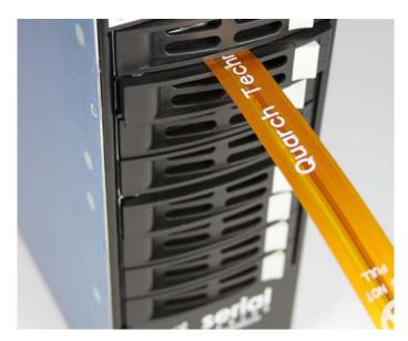
SFF FIXTURES: SUPPORTS SAS, SATA AND NVME (U.3 AND U.2) DEVICES USING SFF-8639 CONNECTORS. SUPPORTS 12V/5V AND 12V/3V3 RAILS VIA A JUMPER SELECTION. SUPPORTS POWER INJECTION SYNC.
