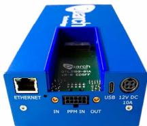
The enclosure is designed to connect to a Serial Cables host card or another MCIO-based controller.
