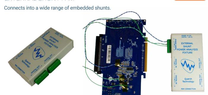
EXTERNAL SHUNT: 4 CHANNELS, SAMPLE RATE 250KS/S, VOLTAGE:  $0-15V\pm(2mV+1\%)$ , CURRENT SENSE:  $10uV-65mV\pm(10uV+1\%)$  DIGITAL CHANNELS: 16 CHANNELS SAMPLE RATE 1MS/S, VOLTAGE RANGE 1.8-5V
