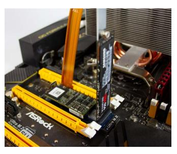
M.2 PAM: ANALOG CHANNELS: 3.3V, VIO\_1V8, SAMPLE RATE 250KS/S, VOLTAGE: 0 - 15V ±(2mV+1%), CURRENT: 0-1mA ±(15uA+1%) 1mA-13A ±(2mA+1%) DIGITAL CHANNELS: CLKREQ#, PERST#, PEWAKE#, SUSCLK, PEDET, ALERT#, SMB\_DATA, SMB\_CLK, LED\_1#, DEVSLP, MFG\_DATA, MFG\_CLK, VIO\_CFG, PWRDIS, PLA\_S3#, PLN# SAMPLE RATE 1MS/S
