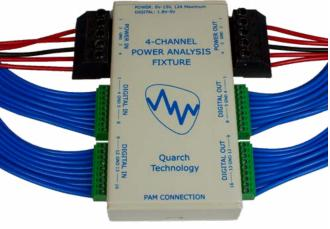
4 CHANNEL: ANALOG CHANNELS: 4 CHANNELS, SAMPLE RATE 250KS/S, VOLTAGE:  $0 - 15V \pm (2mV + 1\%)$ , CURRENT:  $10mA - 13A \pm (10mA + 1\%)$  DIGITAL CHANNELS: 16 CHANNELS SAMPLE RATE 1MS/S, VOLTAGE RANGE 1.8 - 5V
