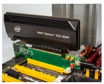
AIC PAM: Analog Channels: 12V, 3.3V, 3.3Vaux, Sample Rate 250KS/s, Voltage:  $0 - 15V \pm (2mV + 1\%)$ , 12V Current:  $100uA - 1mA \pm (10uA + 1\%)$  1mA-13A  $\pm (2mA + 1\%)$ , 3.3Vaux Current:  $0-400mA \pm (10uA + 1\%)$  Digital Channels: PERST#, CLKREQ#, WAKE#, SMBCLK, SMBDAT, Sample Rate 1MS/s
