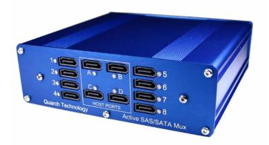
SATA switch with 4 host ports and 8 device ports.
