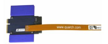
Interposer and flex cable allows power testing within a standard EDSFF enclosure.
