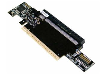
Supports AIC/slot devices up to Gen5 speeds.
