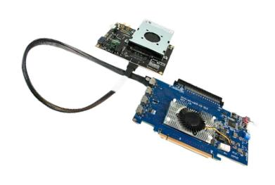
Connect to a compatible MCIO host card, removing the need for adaptors or a U.2 host.
