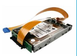
LITE BREAKER: FET SWITCHES ON POWER RAILS, DIGITAL SWITCHING ON SIDEBANDS. HIGH SPEED LANES AND GROUNDS ARE PERMANENTLY CONNECTED. 1MS TIMING RESOLUTION ON HOT-PLUG SIMULATION. BASIC HOT-PLUG ONLY, NO PIN-BOUNCE, DRIVING OR GLITCH. VOLTAGE MONITORING ON SELECTED RAILS.
