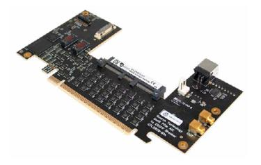
Supports EDSFF devices up to x16. Versions available with lower lane widths.
