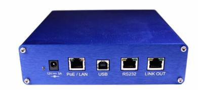
USB, LAN and RS232 Serial control ports.
