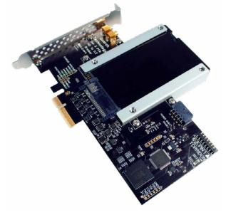
Supports PCIe U.2 drives up to Gen5 speeds in a PCIe x4 slot.
