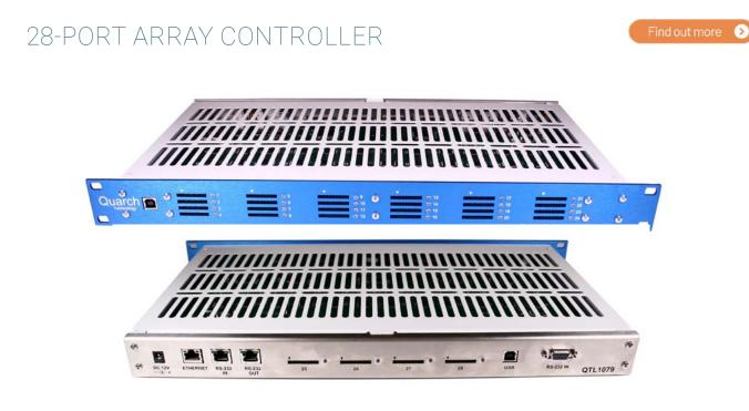
28-PORT CONTROLLER: CONTROLS 28 BREAKER MODULE ACROSS EITHER: DIRECT USB, LAN OR DIRECT RS-232 VIA RS232-D WIRED RJ-45 PORT. 24 PORTS ON FRONT, 4 PORTS ON REAR. 12V 60W SUPPLY. RACK MOUNTS IN 1U. ADDITIONAL USB PORT ON FRONT
