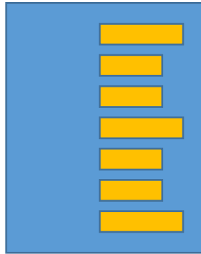
Edge fingers, with two different pin lengths
