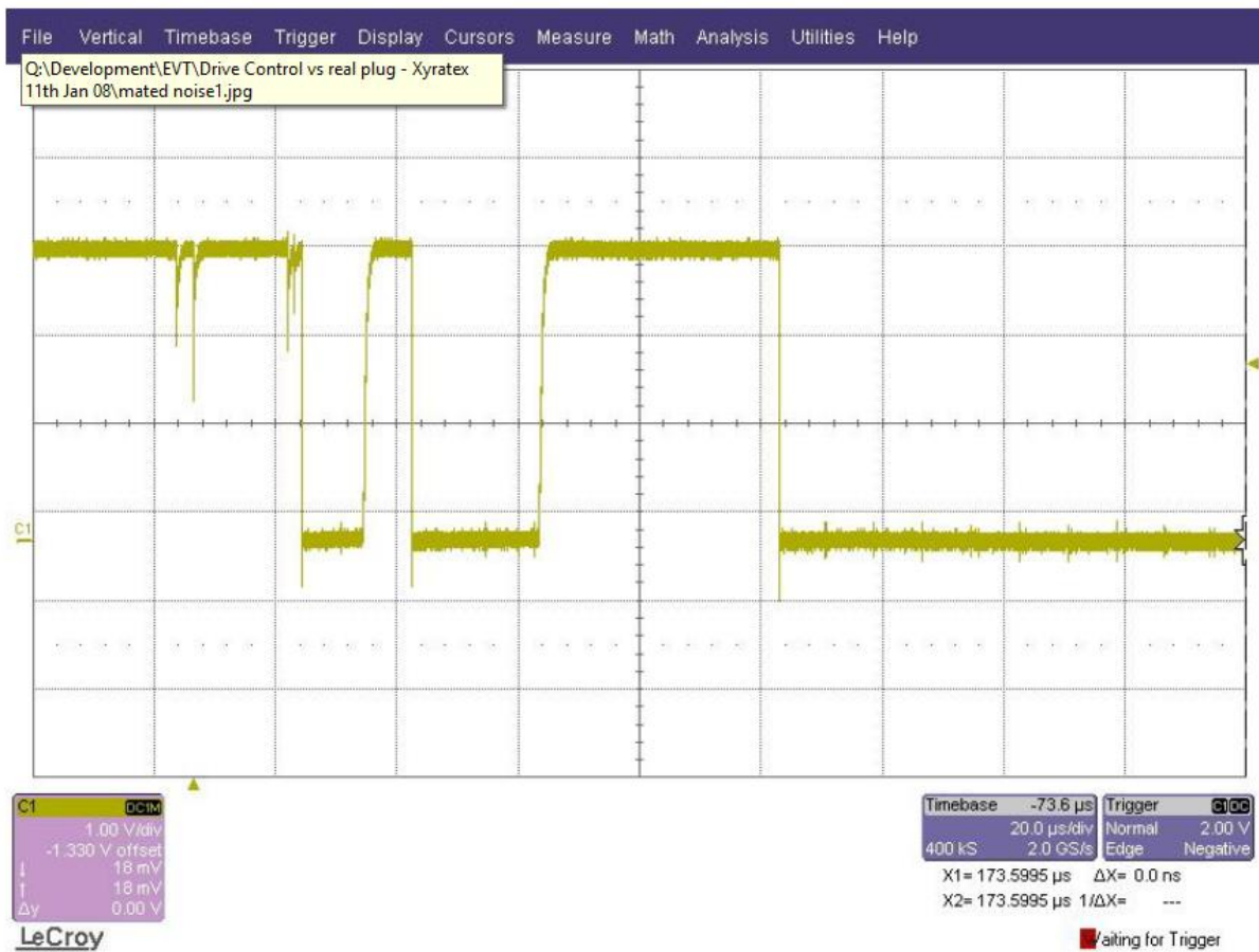
Example of measured pin bounce on drive pull
