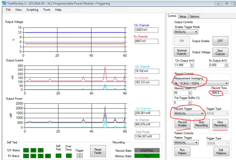
The PPM always samples at 250kS/s. The TestMonkey 2 GUI is used to set up the PPM to average 2048 samples to make each recorded value and to record each averaged value for 400 seconds starting when the Record Enable button is pressed.
